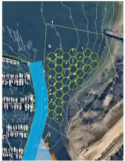
Figure 10 – Proposed Mooring Ground Arrangement Grid (Aerial image: Nearmap 29/10/2021)
